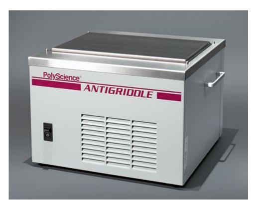
Applies an instant deep freeze **How it works:** The Anti-Griddle maintains a constant temperature of  $-30^{\circ}$ F by pumping a refrigerant through a compressor to remove heat from the smooth steel surface. The result: Liquids, creams and gels get a frozen crust in 30 to 90 seconds, while staying creamy inside. **On the menu:** Crème-anglaise lollipops, whipped-cream pancakes—A.W.
