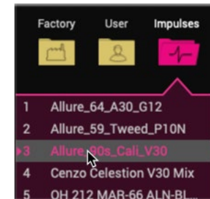
Just double-click on any IR within the Impulses list to load it in the IR block
