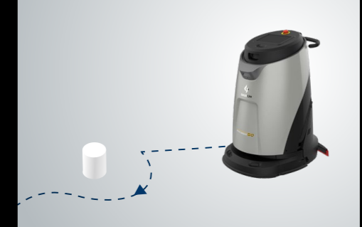
REPLANS THE PATH WHEN BLOCKED BY OBSTACLES
