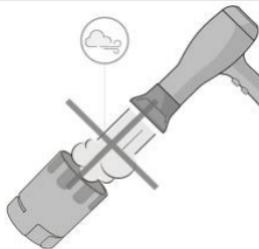
Correct operation of the turbine is guaranteed only if it is "clean" and free of foreign objects that affect its movement. The presence of dust or foreign bodies (such as hairs, sputum etc.) could slow or block the moving parts of the turbine and make the result less accurate, or damage the turbine itself.
