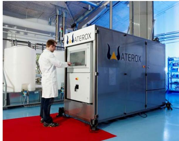
*Aquarden's Waterox system breaks down all hardly-degradable organic pollutants completely in a few seconds without adding any chemicals.*
