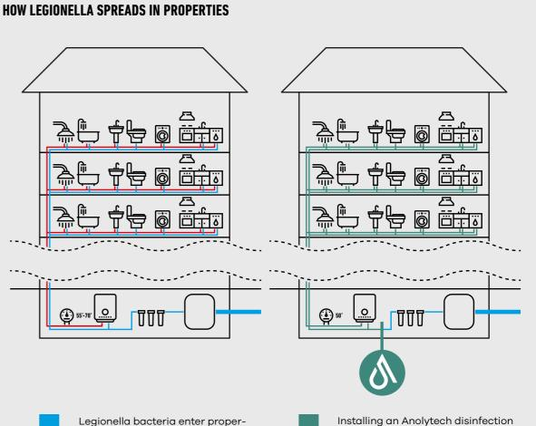
ties via the incoming water supply and then spread through the cold water pipes.
