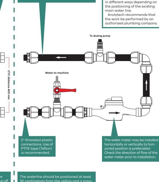
Existing main waterline should be cut and 3 shut-off valves **"bypass"** fitted. This will mean that the water will never need shutting off during maintenance of the water meter and dosing point, or troubleshooting.
