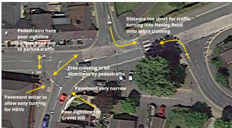
Figure 36. Pedestrian hazards at East Hamlet junction
