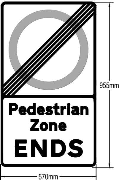
Example zone exit sign
